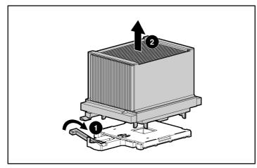
Figure 1-17: Removing a processor
